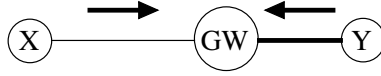
Figure 1.1: An example of MAC unfairness due to capture effect in a mesh network.
