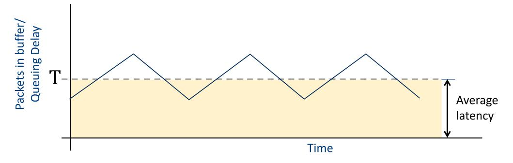
Throughput is maximum because buffer is always filled
