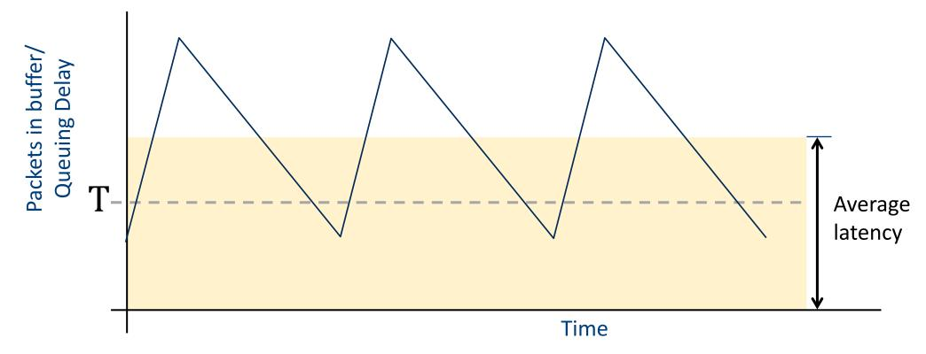
By adjusting the parameters,  $k_{\rm f}, k_{\rm d}$  and T, we can change the shape of the sawtooth.
