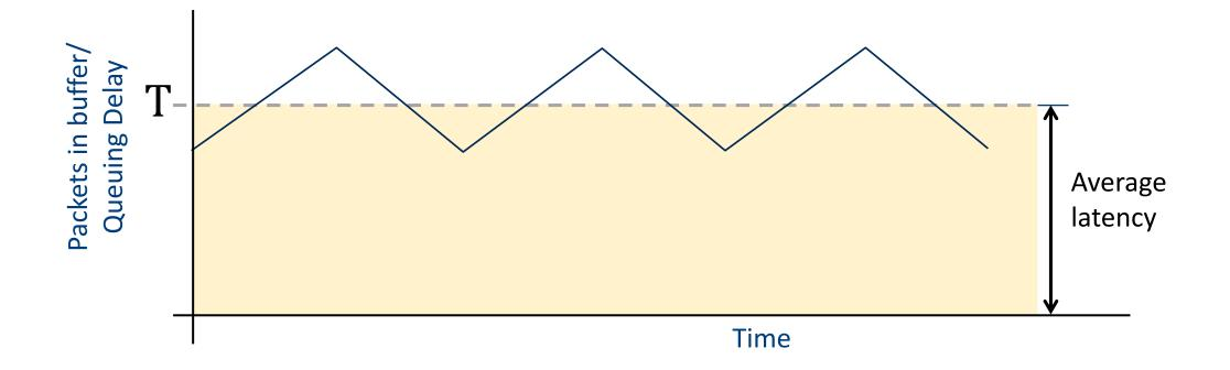
Throughput is maximum because buffer is always filled
