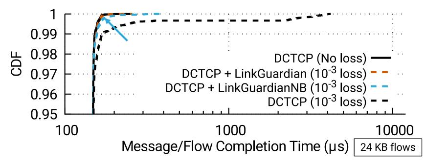
LinkGuardianNB: nearly the same improvement, even without maintaining pkt order! <u>TCP flows are short:</u> reduction in cwnd (due to out-of-order) has minimal impact! (more detailed analysis in the paper)
