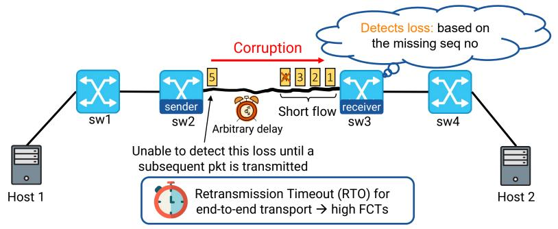
Goal #3: Detect and recover tail packet losses (as quickly as possible)
