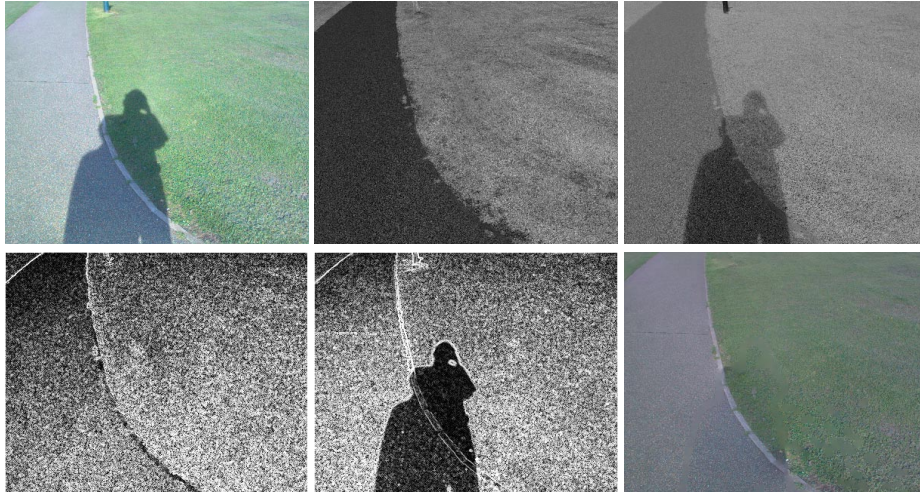
Fig. 1. (a): Original image. (b): Grey-scale illuminant-invariant image. (c): Grey-scale non illuminant-invariant image. (d): Edge map for invariant image. (e): Edge map for non-invariant image. (f): Recovered, shadow-free image.
