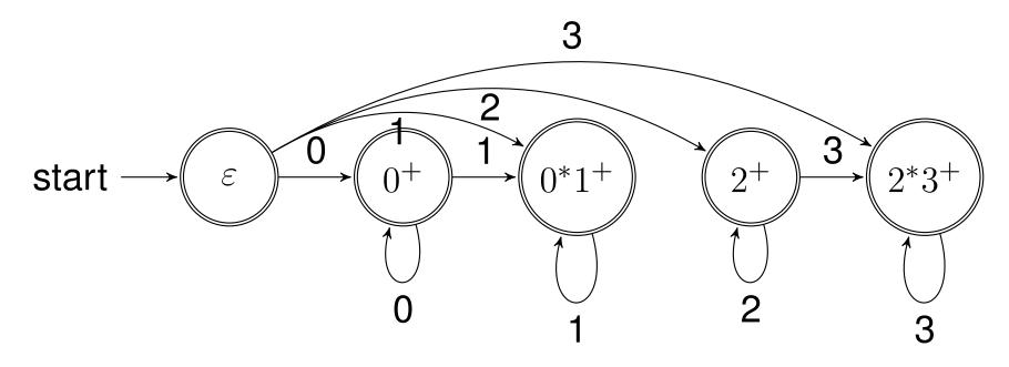
One new starting state is added and the transitions from old starting states to successor states are now done from the new starting state directly.
