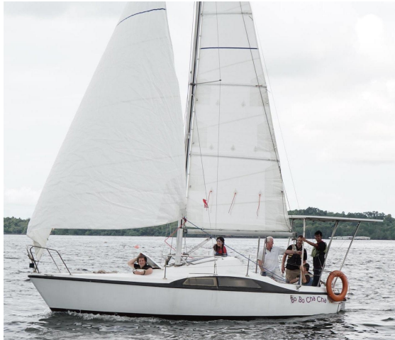
Figure 6: Pocket cruiser Bo Bo Cha Cha (Maxi 77) with a crew of six, operating in Singapore waters in light winds in wind/electric hybrid mode
