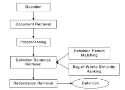
Figure 1. Architecture of the definitional QA system.
