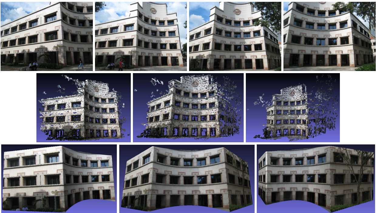
Fig. 9 Reconstructed mesh models of building 1. (Row 1) Sample images from various views. (Row 2) Point cloud recovered by PMVS and (Row 3) reconstructed textured mesh model at various viewing angles.
