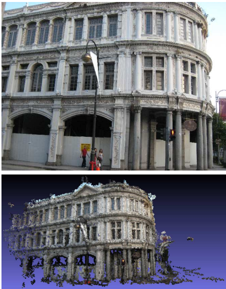
Fig. 1 Recovery of 3D point cloud. (Top) A sample input image of a building. (Bottom) Recovered 3D point cloud.
