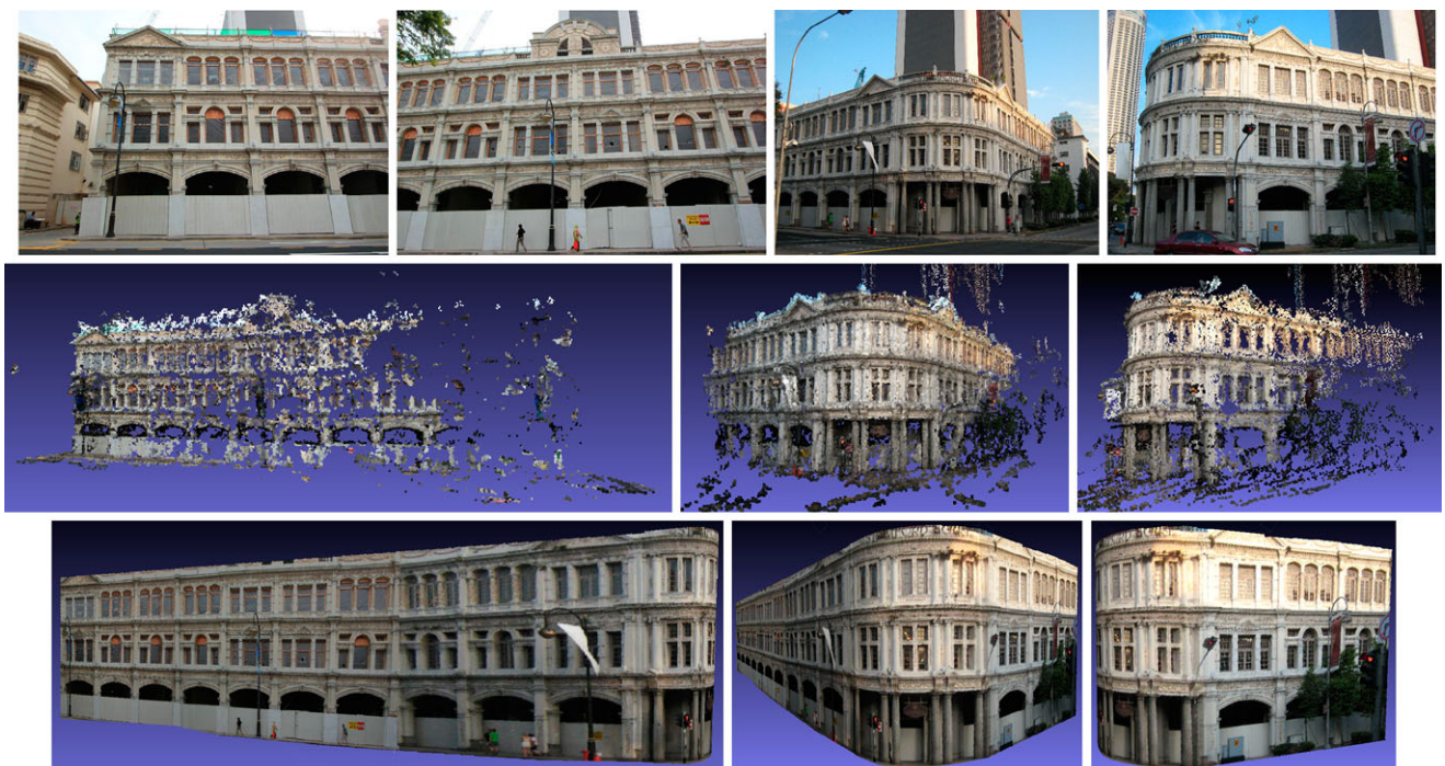
Fig. 6 Reconstructed mesh models of building 2. (Row 1) Sample images from various views. (Row 2) Point clouds recovered by PMVS and (Row 3) reconstructed textured mesh model at various viewing angles
