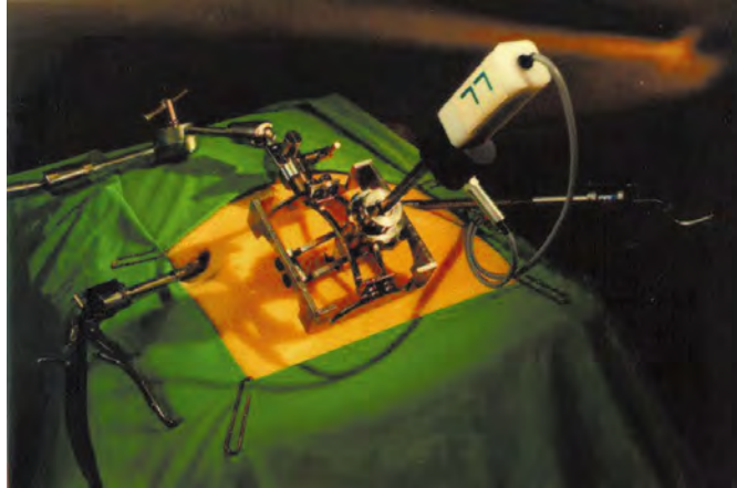
Figure 3.1: The instrument box for the surgeons to input surgical operations to the system [37].
