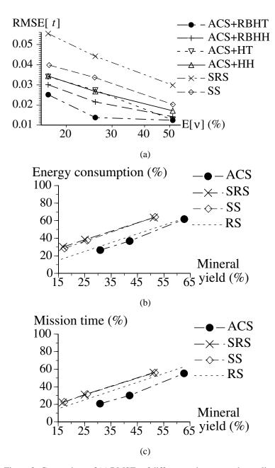
Figure 3: Comparison of (a) RMSEs of different estimators and sampling strategies, (b) energy consumption of different sampling strategies, and (c) mission time of different sampling schemes.
