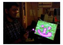
Figure 7: A tracked "paintbrush" painting on a tracked cuboid. The tracker information allows the computer to generate the correct images to illuminate the tip of the "brush" and the cuboid by the projectors.
