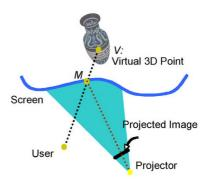
Figure 2. Geometric relationship for displaying virtual object. The user could be static or moving.
