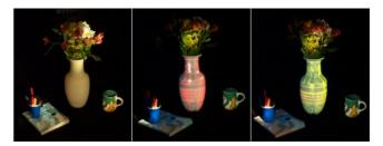
Figure 6: (Left) The underlying physical object is a white diffuse clay vase. (Middle and right) View-dependent effects, such as specular highlights, can be generated by tracking the user's location and projecting images on the physical vase.
