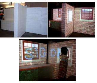
Figure 1: (Top-left) The physical model is made of styrofoam blocks, and it approximates the geometry of the virtual environment. (Top-right) Perspectively-correct imagery of the scene is generated in real-time and projected onto the blocks. (Bottom) The user can interact with the surfaces using a virtual spray paint.
