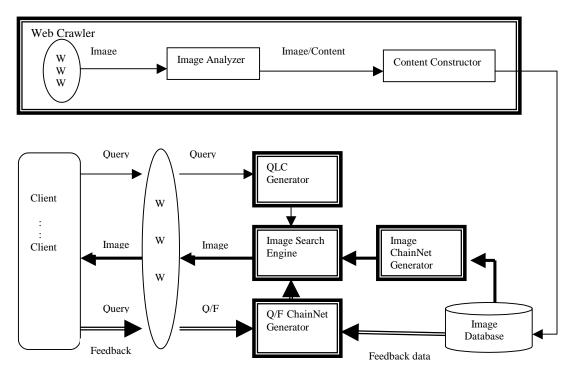
Figure1: Overall system structure in client-server form.
