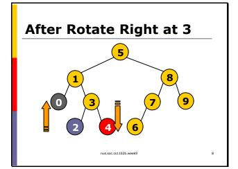
Rotation changes the heights of nodes. In this example, the depth of node 4 increases by 1. The depth of node 0 decreases by 1. The depth of node 2 remains unchanged.
