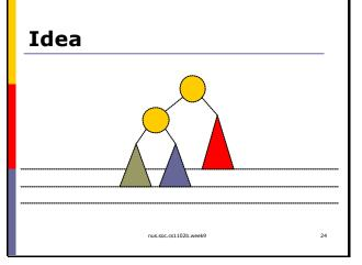
We can insert into the red subtree, blue subtree, or gray subtree. Insertion in red subtree never violates the AVL tree property. But insertion into blue and gray subtree \_may\_ cause a violation.
