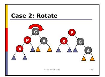
If X's uncle is black, and X is a left child, we do a single right rotation around its grandparent, and then do a color flip. After this, node that the parent is black, so we do not need to fix the tree any further (unlike case 1).
