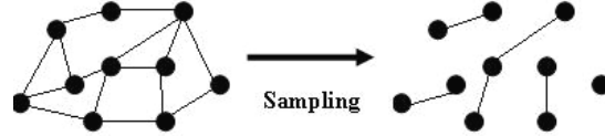
Fig. 1. Sampling on the network: each link is picked randomly with a probability \rho to be included in the subnet.
