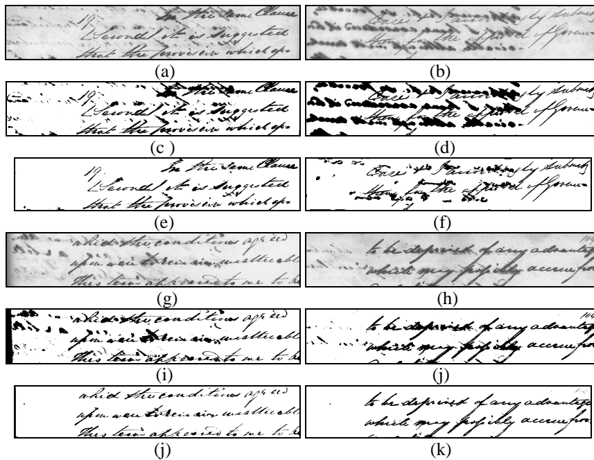
Figure 16. (a), (b), (g), (h): original test images; (c), (d), (i), (j): the binary microfilm copies of (a), (b), (g), (h) separately; (e), (f), (j), (k): the binary images of segmentation results by the proposed algorithm of (a), (b), (g), (h) respectively, Ostu's threshold method 4 .
