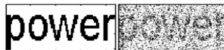
Figure 2 Left: Test image ideal binarization; Right: Original test image corrupted by Gaussian ( \sigma = 1.0 ) and impulsive ( p=0.1 ) noise.
