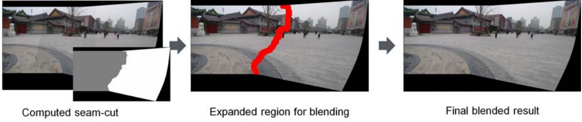
Figure 4. This example shows our blending procedure where a seam-cut is first computed, followed by blending about the seam.
