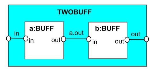
Suppose we want to put the two cells together in the above fashion. What will be the process equation describing the TWOBUFF process.
