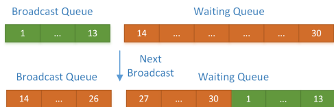
Figure 4: How the broadcast queue works.
