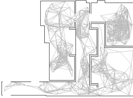
Figure 10: The office floorplan used for sensor network simulation. Dark lines are the walls of the building and light-colored lines represent the graph edges between nodes. Each edge represents a distance measurement that a node can perform. Measurements cannot be taken through walls.
