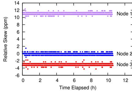
(b) Clock skew measured at 1-min intervals between the sending node receiving nodes.
