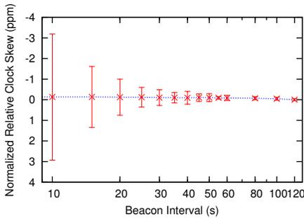
(a) Mean and variance of clock skew measured at one node using different time intervals.
