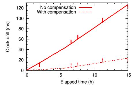
(c) Amount of clock drift between two nodes with and without clock drift compensation.
