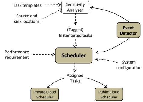
Figure 3. Architecture of hybrid cloud video surveillance system.
