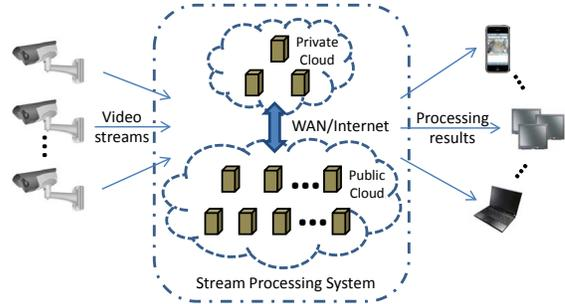
Figure 1. System model for hybrid cloud video surveillance.
