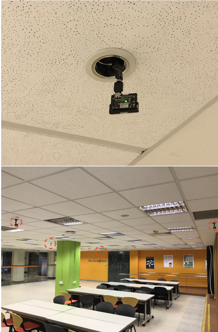
Fig. 2: Motes as deployed in the building.
