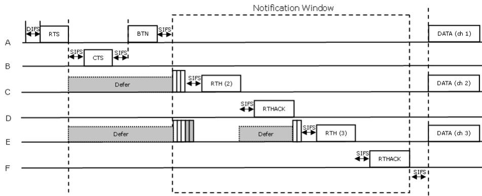
**Figure 1. Operations of AMCM with 3 competing traffic flows (A→B, C→D, E→F)**
