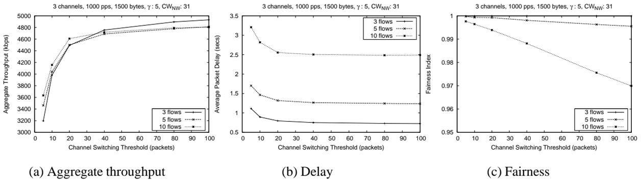
Figure 9. WLAN: Impact of  $CST$
