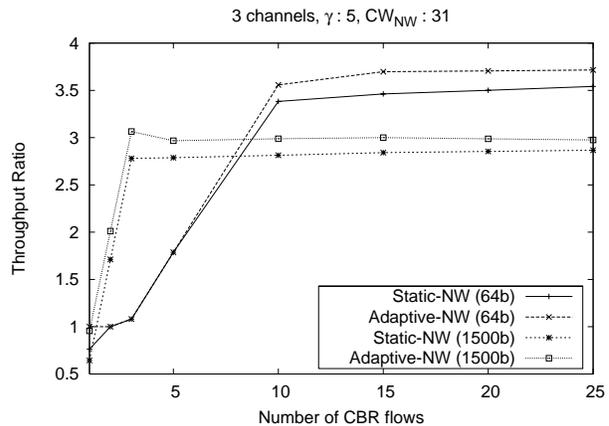
**Figure 4. WLAN: Impact of number of traffic flows**
