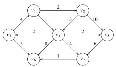
Shortest path from  $v_1$  to  $v_6$  has a cost of 6 and goes from  $v_1$  to  $v_4$  to  $v_7$  to  $v_6$ .
