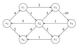
path from  $v_5$  to  $v_4$  has cost 1 but a shorter path exists:  $v_5$  to  $v_4$  to  $v_2$  to  $v_5$  to  $v_4$  This is a *negative cost cycle*
