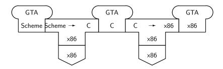
Compiling "GTA" from Scheme to C to x86 machine code
