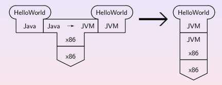
Compiling "HelloWorld" from Java to JVM code, and running the JVM code on a JVM running on an x86
