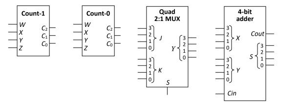
Given the above 4 components, you are to employ block-level design to design the converter, without using any additional logic gate or other devices. You may observe that if A = 1, then the output FGH is simply the number of 1s in the input ABCD. You are to make your own observation for the case when A = 0.
