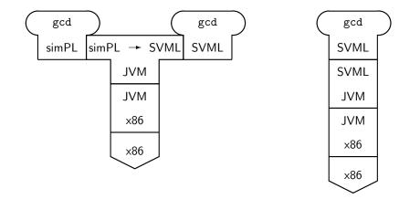
**Example 8.11** Using the compiler simple and the emulator simpl, both written in Java, we can execute a given simPL program gcd.simpl as follows:
