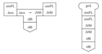
Instead of directly executing the instructions, we can instead store the instruction array in a file (in Java easily done using an ObjectOutputStream). This amounts to a simPL compiler, which translates simPL files to SVML files.
