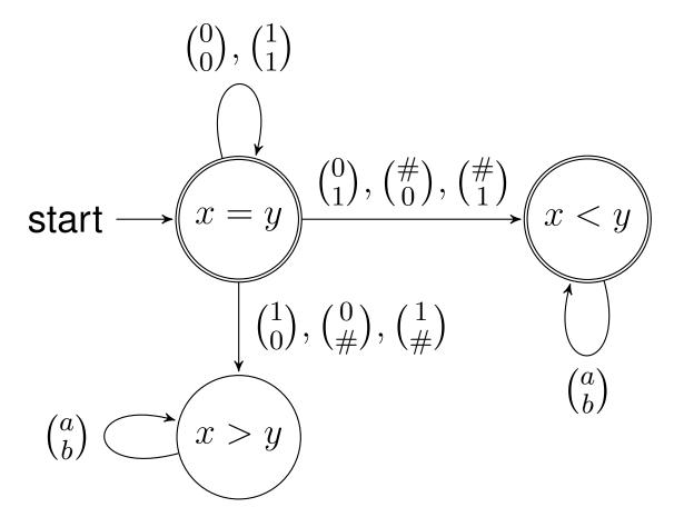
Here  $\binom{a}{b}$  on an arrow means that the automaton always goes this way.
