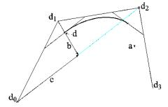
**Fig 6.** The power basis form of a cubic curve  $(a*t^3 + b*t^2 + c*t + d)$  has an interesting relationship to the geometry of the uniform B-spline control vertices. For instance, b is the vector from d to half way between d and d
