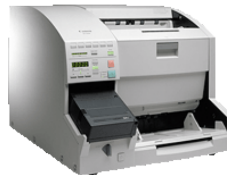
A high speed scanner, 1.2 pps at 200 dpi
