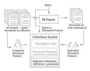
Figure 2: CENTRIFUSER architecture.
