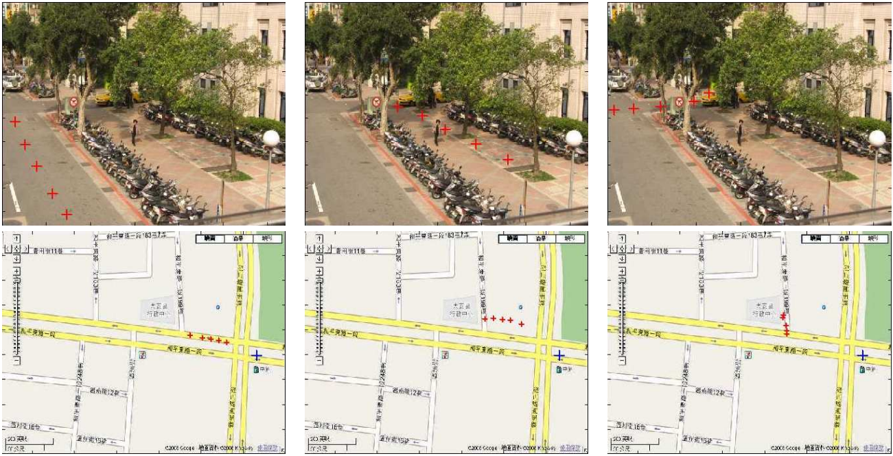
Figure 8: 2D-to-3D position mapping test results. (Top) Input 2D positions indicating human’s walking paths. (Bottom) Mapped 3D positions in the city map.
