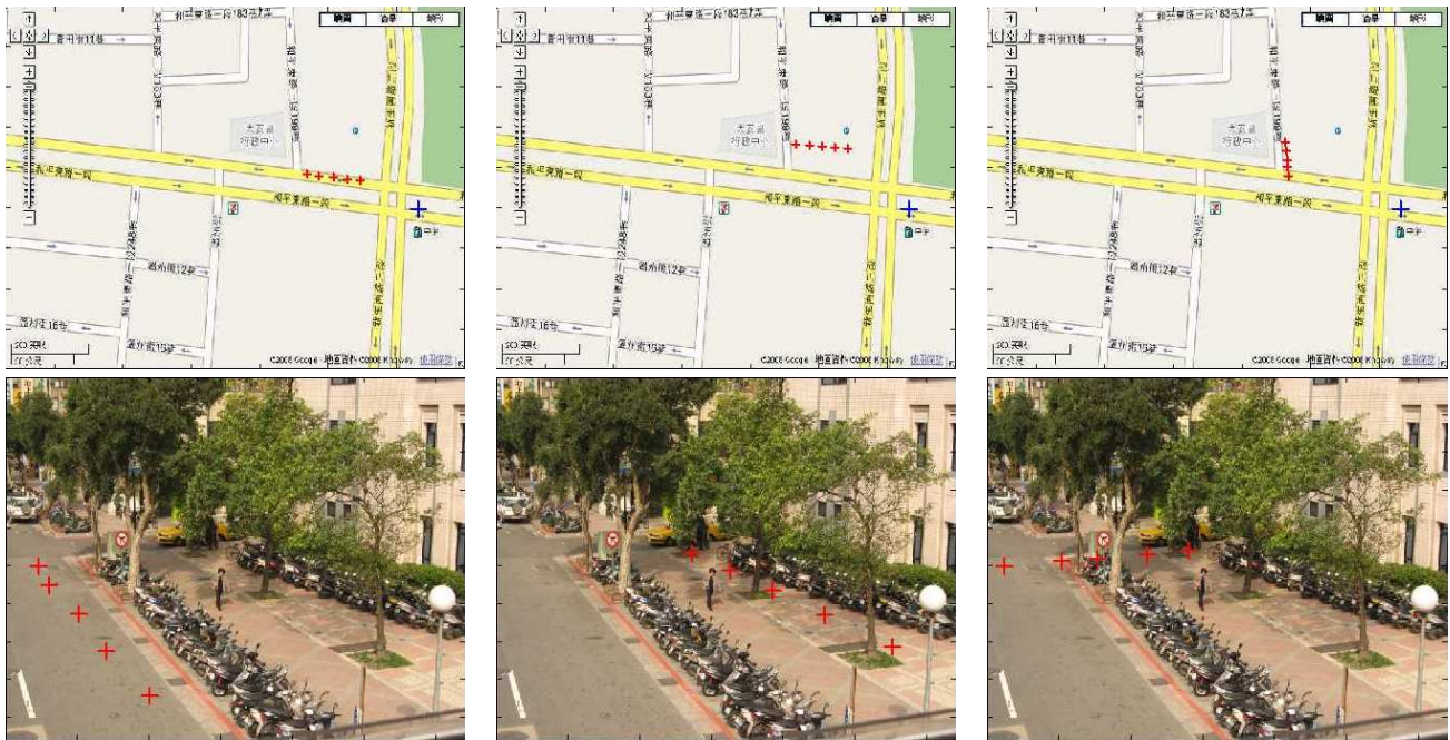
Figure 7: 3D-to-2D position mapping test results. (Top) Input 3D positions indicating human's walking paths. (Bottom) Mapped 2D positions in the camera view.
