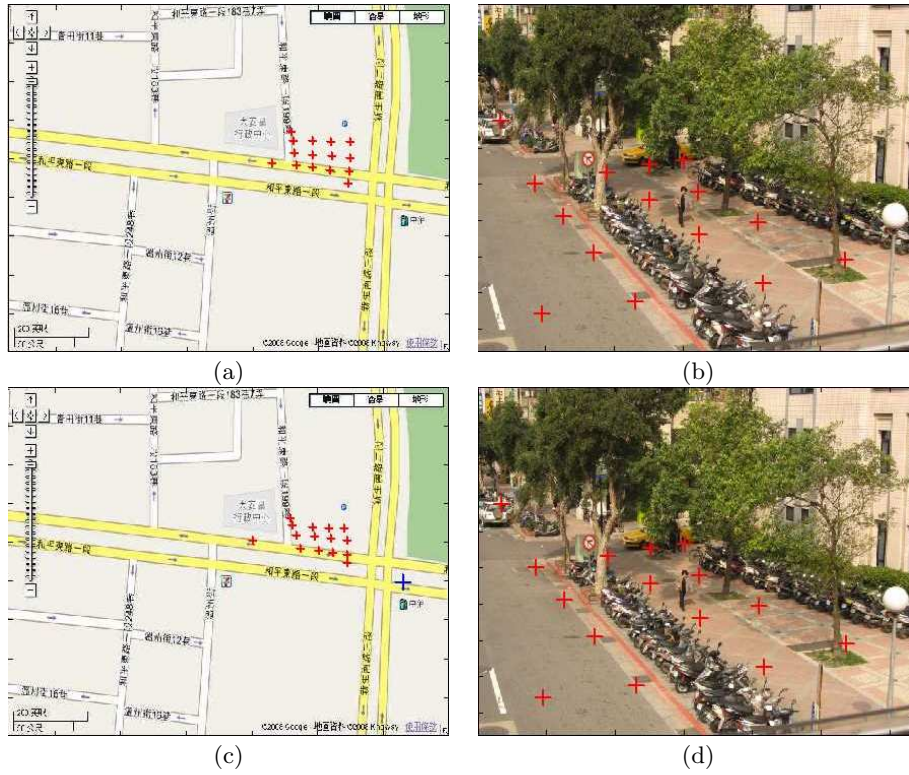
Figure 10: Mapping positions between city map and camera view. Corresponding points (red crosses) are manually marked in (a) city map and (b) camera view. (c) 2D-to-3D mapping results. Blue cross: recovered camera position. (d) 3D-to-2D mapping results.
