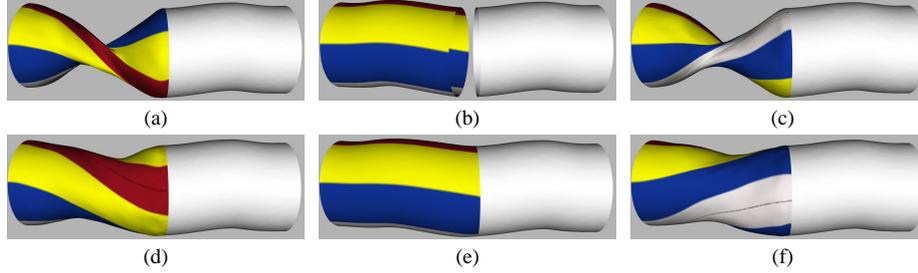
**Figure 2.** Test case 1: Joining of two relatively straight blood vessel models. The left blood vessel is shaded in color to visualize torsion. (a, c) Large amount of torsion. (b) Initial configuration. (d, f) Medium torsion. (e) Minimum torsion configuration found by the algorithm.
