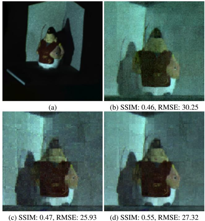
**Fig. 1.** Dual photography. (a) Camera view. (b) Dual image directly reconstructed from 16000 samples, which is not practical. (c) Dual image progressively reconstructed from only 1000 samples using our method with 64 basis dual images. (d) Dual image reconstructed with settings as in (c) but from 1500 samples. Haar wavelet is used for the reconstruction.
