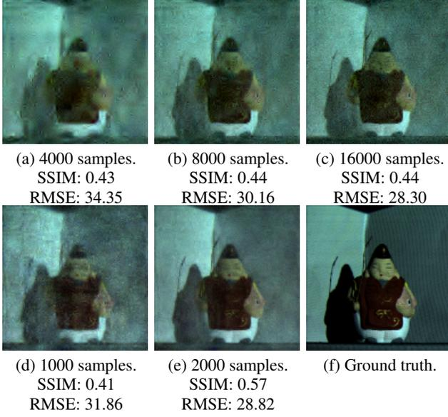
**Fig. 2.** Comparison between direct and progressive reconstruction. Dual image (a), (b), and (c) are from direct reconstruction. Dual image (d) and (e) are from progressive reconstruction with 64 basis dual images. (f) Ground truth is generated from light transport from 16000 samples by inverting the circulant measurement matrix. Daubechies-8 wavelet is used for the reconstruction.
