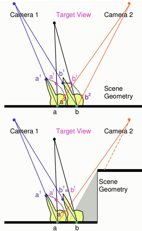
**Figure 1.** (Top) The blending function at each scene point can be expressed as a weighted combination using local information such as the angles between the target ray and the corresponding source rays. The yellow region indicates local radiance. (Bottom) In the case of view-dependent surface reflectance, and in the presence of depth discontinuities, the neighboring scene points may have very different contributions from the source images.
