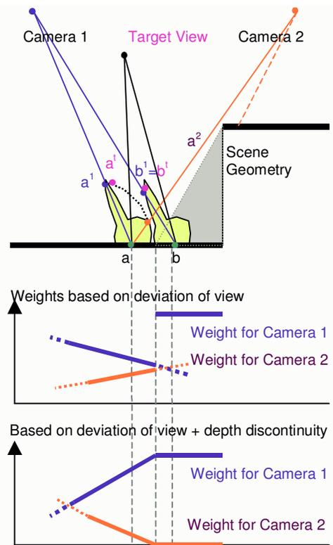
**Figure 2.** (Top) The weighted combination  $a^t$  is very similar to  $a^1$  if feathering across depth discontinuity is considered. (Middle) The traditional feathering based on local information has a gap in the assigned weights. (Bottom) Our method considers depth boundaries to ensure smoothness.
