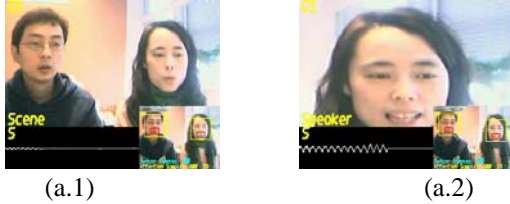
(a.1) Sound in the audio stream triggers the lip motion detector in C1 . (a.2) C2 focuses on the speaker's region detected by lip motion detector.
