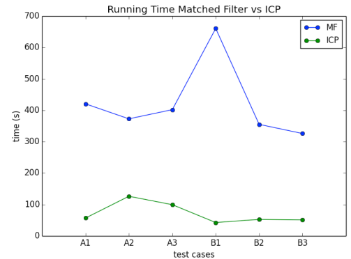
Figure 4.4: Running time of matched filtering (blue) and ICP (green).
