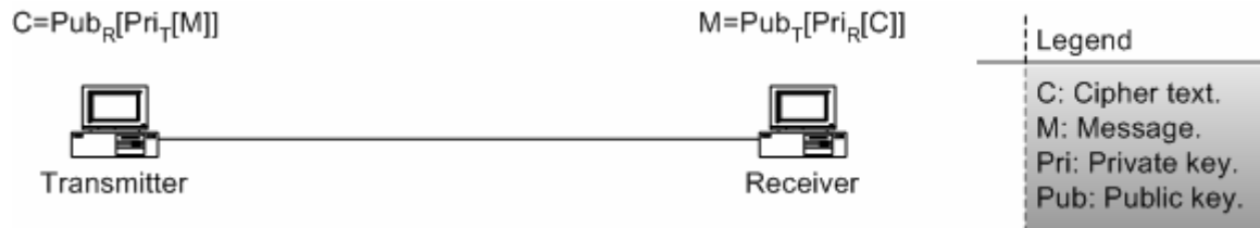
Figure 6.2: Authentication and confidentiality in asymmetric ciphers. Adapted from [43].
