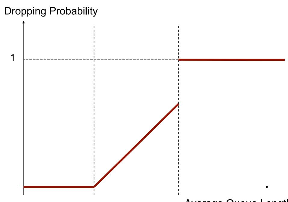
foreach incoming packet X calc average queue length if min<sub>th</sub> < average < max<sub>th</sub> calc p drop X with probability p else if average > max<sub>th</sub> drop X
