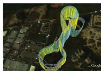
Figure 2. DCS tracking (yellow) and stock autopilot tracking (blue) on racetrack flight path.
