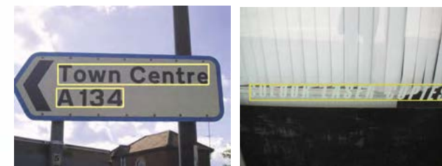
Figure 10: Sample scene text detection results. The yellow bounding boxes indicate the text positions detected by our technique
