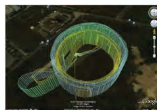
Figure 3. DCS tracking (yellow) and stock autopilot tracking (blue) on circular flight path.
