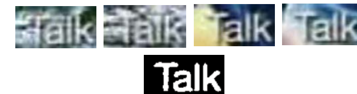
Figure 13: Sample video text recognition result. The left hand side shows a few instances of the same word over time. The right hand side shows the integrated and binarized text image. By using temporal information, the final recognized string is correct, despite the low quality of the individual text instances.
