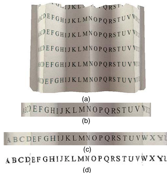
Figure 5. (a) Folded paper (b) Portion of the distorted image (c) Restored result (d) Restored result (Binary)
