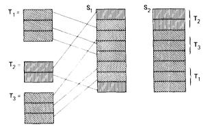
Fig. 4. Three schedules for  $T_1$ ,  $T_2$  of Fig. 1.  $S_1$  is equivalent to serial schedule  $S_3$  and hence is consistent.  $S_2$  is inconsistent.
