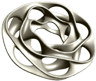
Fig. 1 The layer peeling algorithm is able to reconstruct surfaces from point sets of complex topology.
