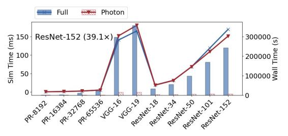
kernel execution time (left y-aixs with lines); Wall time (right y-axis with bars)
