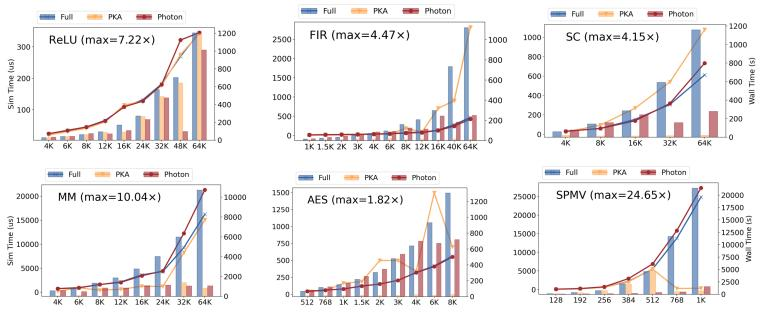
kernel execution time (left y-aixs with lines); Wall time (right y-axis with bars)
