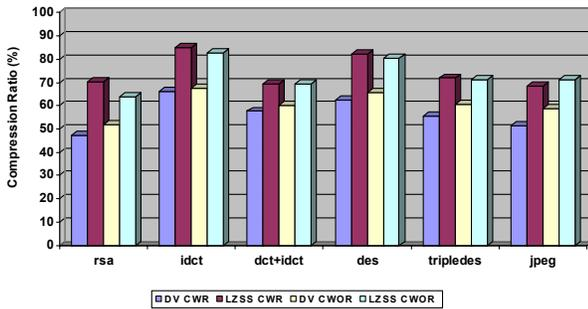
Figure 5. Intra-bitstream Compression with DV and LZSS
