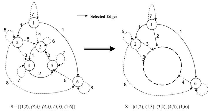
Figure 3. Tree Generation for Inter-Bitstream CWR
