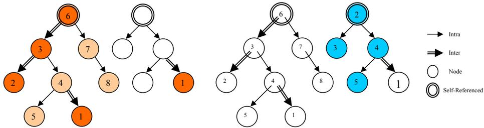
Figure 4. Tree Traversal for Inter-Bitstream CWR
