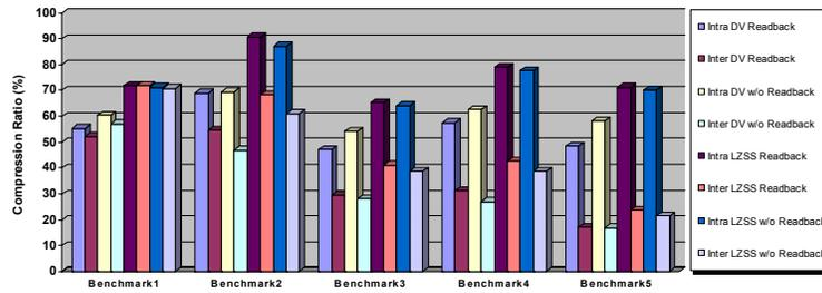
Figure 6. Compression Ratio for Inter-Bitstream DV and LZSS Schemes
