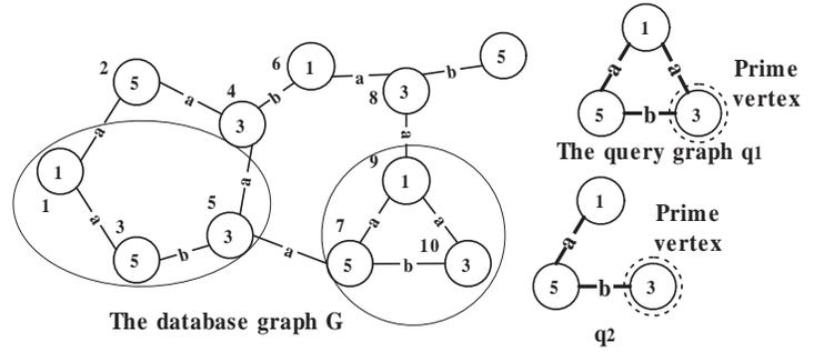
**Figure 6: Matching  $q_1$  based on its subgraph  $q_2$**
