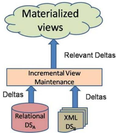
**Figure 5. Using Deltas in Native format for Incremental View Maintenance**
